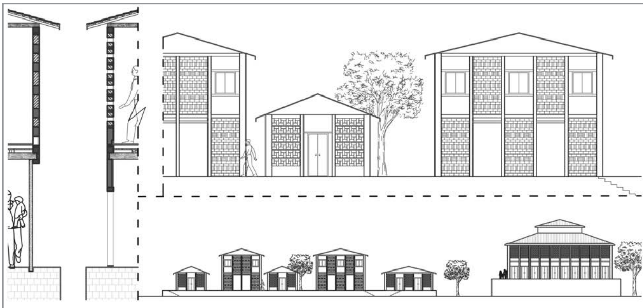
Output 6: SDS and FDP inserts for vertical surfaces and perforations - concrete for wall panels, masonry blocks and jaali walls 13
