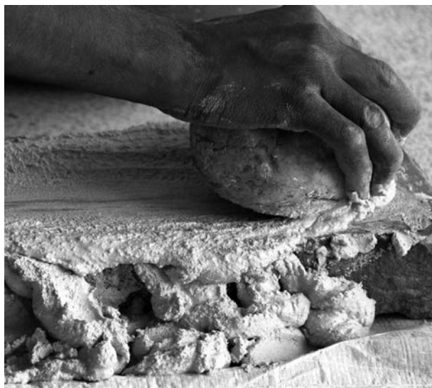
Stone grinding of lime mortar
