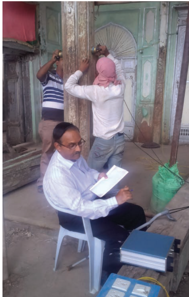
Testing timber using UPV meter. Source: Jeernodhar Conservators pvt. Ltd. project in Gulbarga, Karnataka
