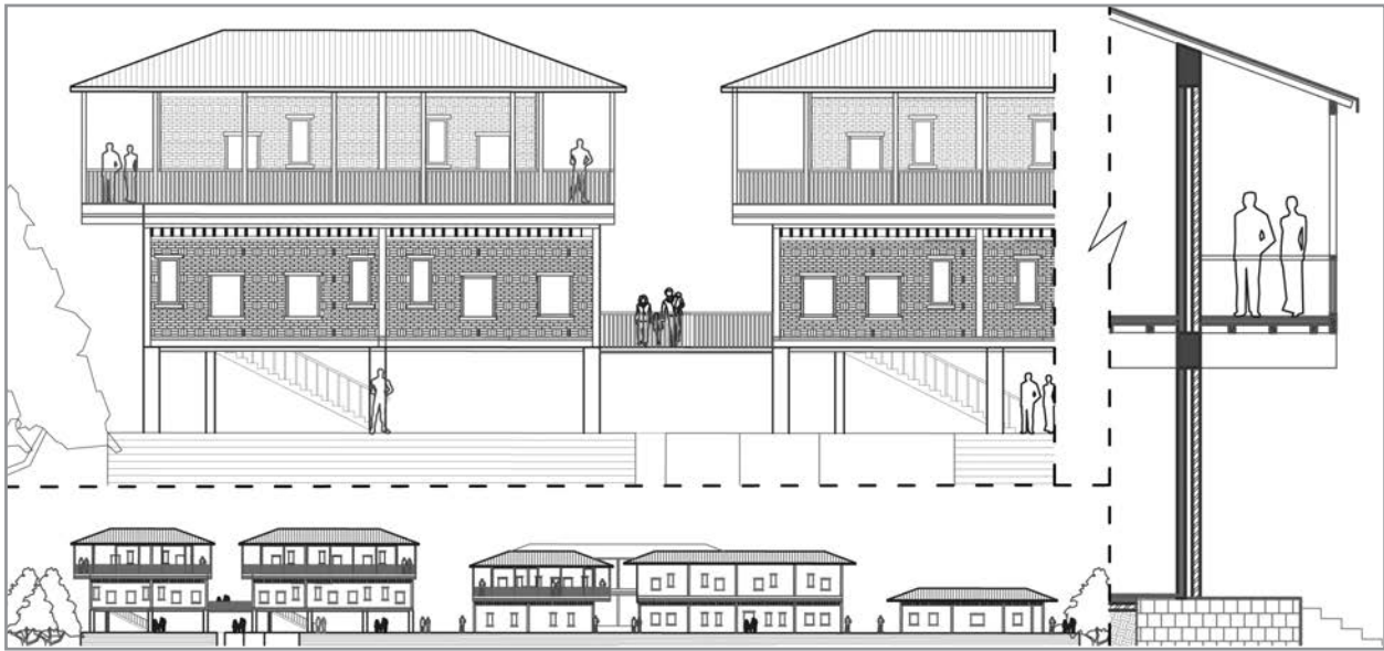
Output 7: FDS, FDP and CI inserts for volumes and vertical surfaces: concrete for beams, concrete blocks for cavity walls and plain cement concrete for floor infill 14
